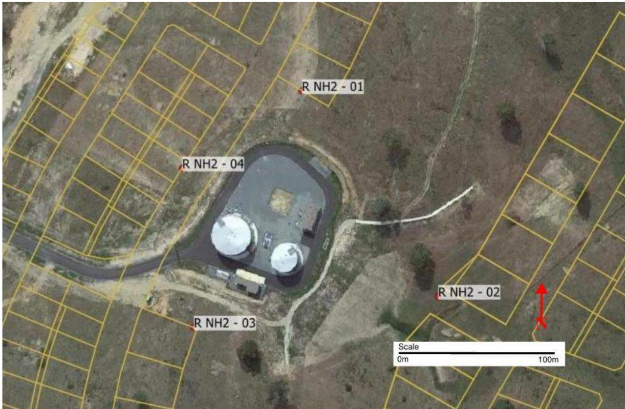
Figure 6.23 Assessed receivers for Stage D operational noise at the Permanent Reservoir site (WSP, 2020)
