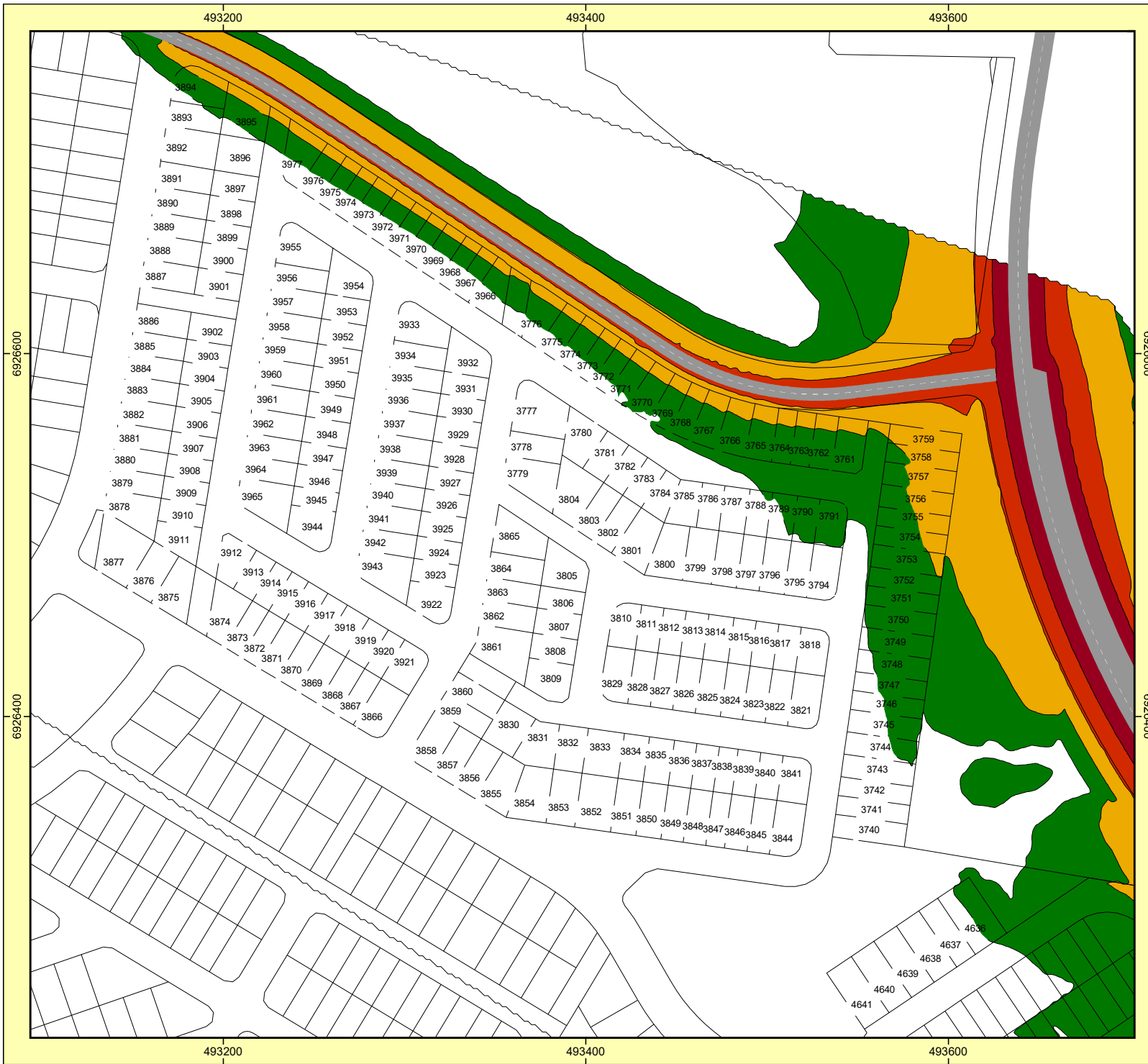
Figure 6 - QDC MP4.4 Noise Categories 2041 Road Traffic Noise Levels Ground floor noise prediction at 1.8m above the ground without noise barriers
