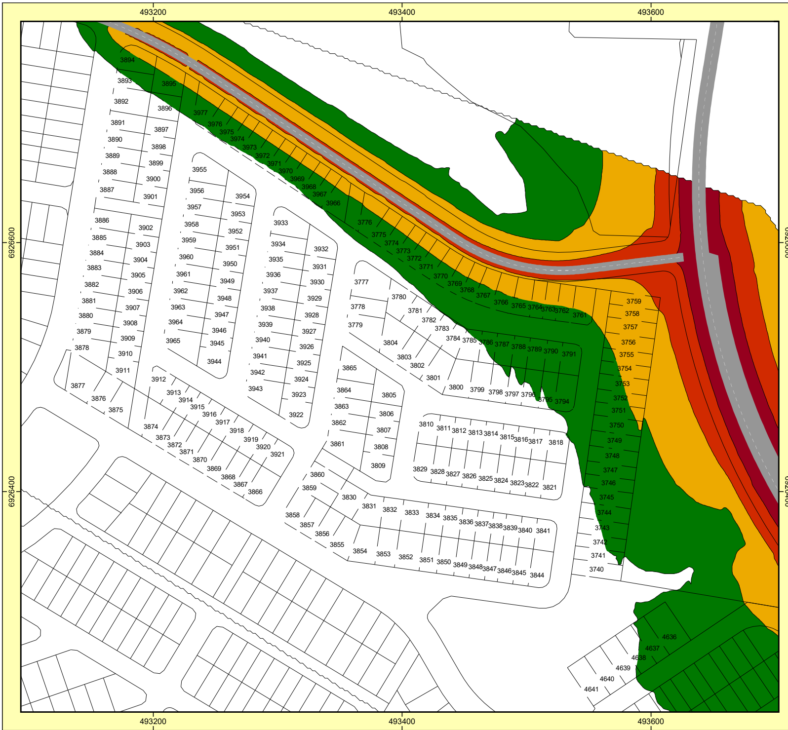
Figure 8 - QDC MP4.4 Noise Categories 2041 Road Traffic Noise Levels First floor noise prediction at 4.6m above the ground without noise barriers
