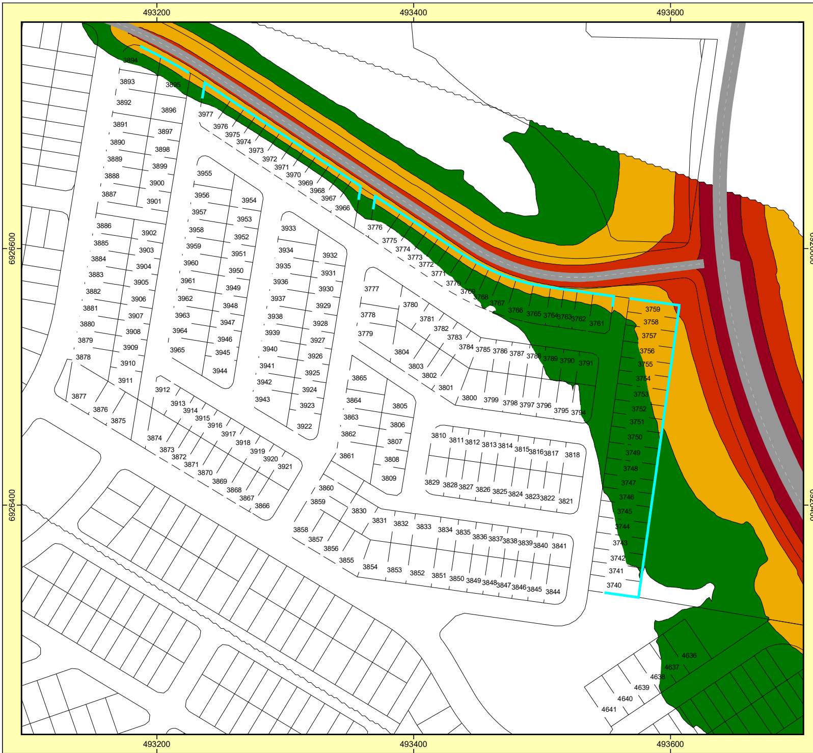
Figure 9 - QDC MP4.4 Noise Categories 2041 Road Traffic Noise Levels First floor noise prediction at 4.6m above the ground with 2.0m high noise barriers
