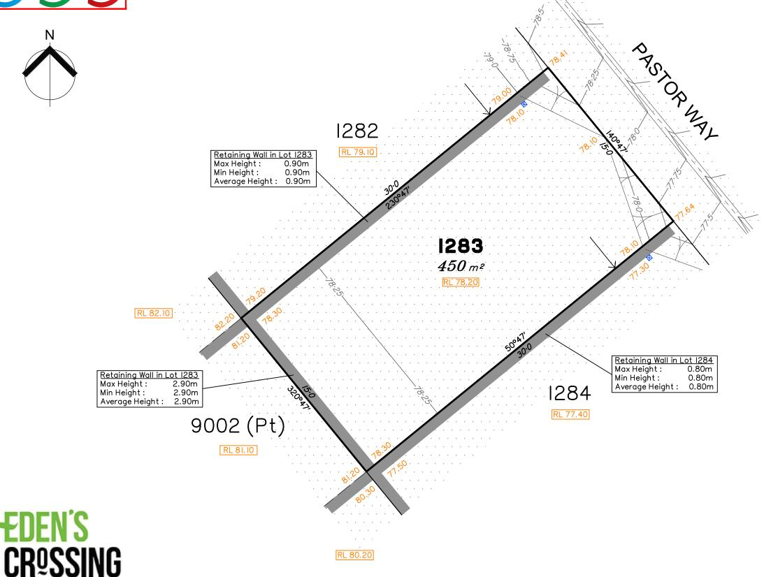
**LEGEND** Area of Cut Area of Fill **Design Contours** Depth of Fill Top of Batter Toe of Batter Retaining Wall Preferred Earthworks Pad Level Finished Surface Design Level Optional Built to Boundary Wall 300mm x 300mm Subsurface Drainage Pit (indicative location) (Not all items in this legend may be relevant to the lot shown on this plan)
