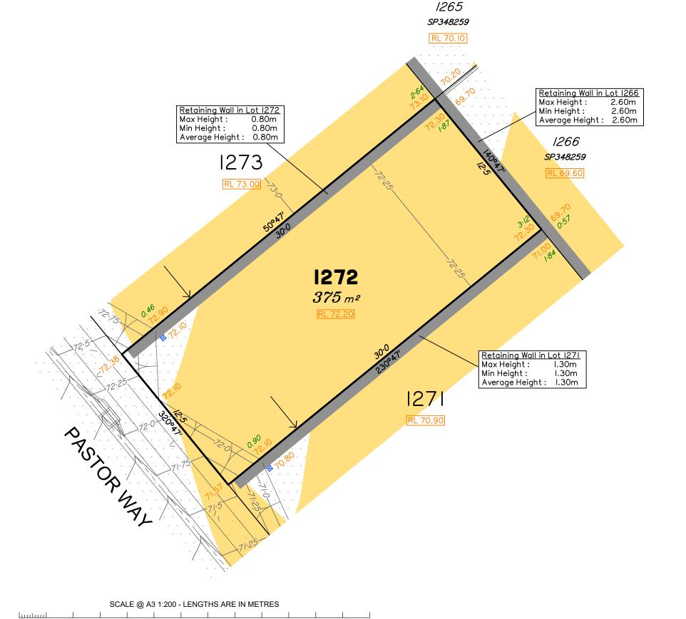
**LEGEND** Area of Cut Area of Fill **Design Contours** Depth of Fill Top of Batter Toe of Batter Retaining Wall Preferred Earthworks Pad Level Finished Surface Design Level XX.XX
