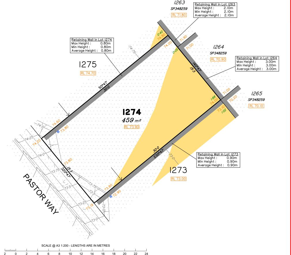
**LEGEND** Area of Cut Area of Fill **Design Contours** Depth of Fill Top of Batter Toe of Batter Retaining Wall Preferred Earthworks Pad Level Finished Surface Design Level Optional Built to Boundary Wall 300mm x 300mm Subsurface Drainage Pit (Not all items in this legend may be relevant to the lot shown on this plan)
