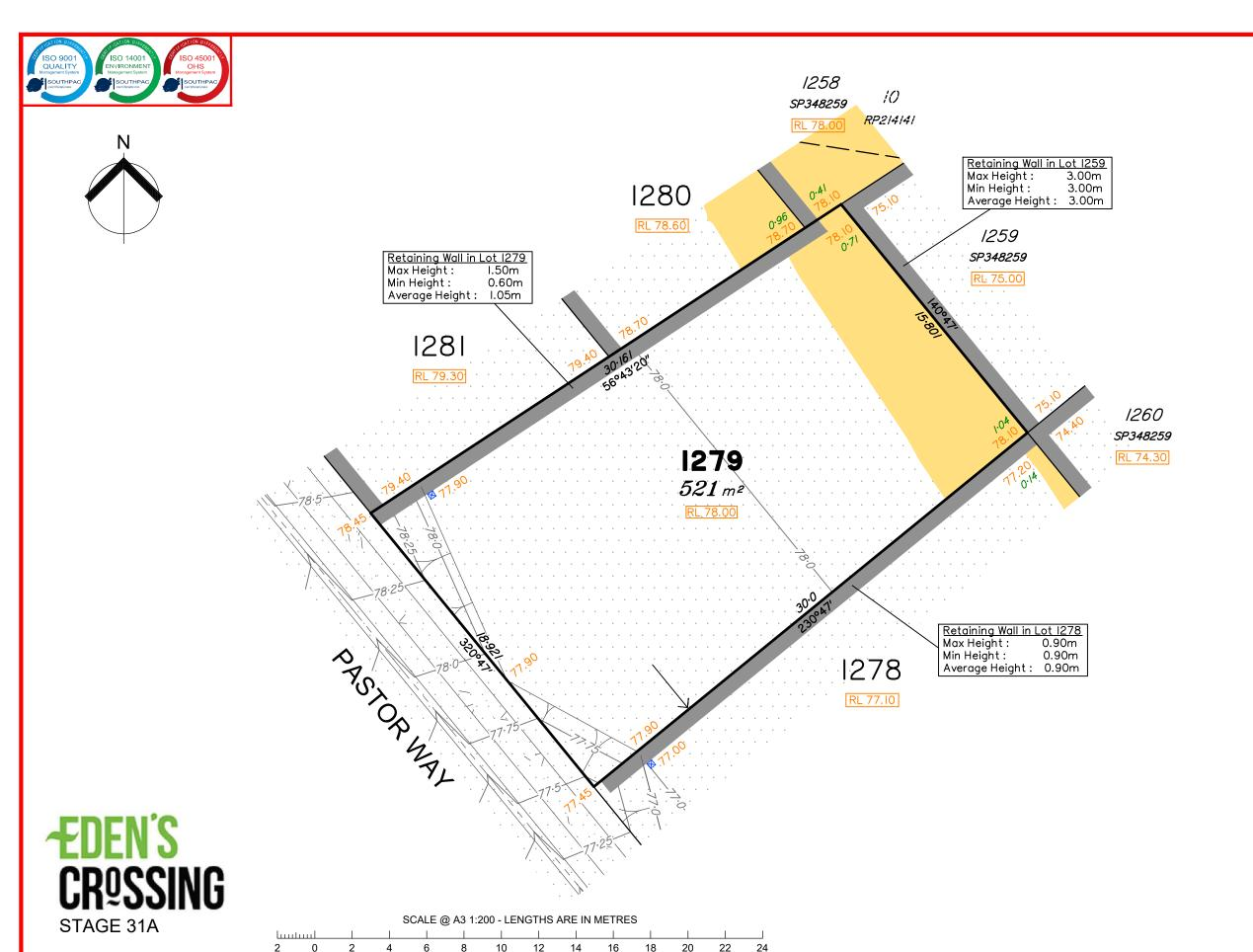
**LEGEND** Area of Cut Area of Fill **Design Contours** Depth of Fill Top of Batter Toe of Batter Retaining Wall Preferred Earthworks Pad Level Finished Surface Design Level Optional Built to Boundary Wall 300mm x 300mm Subsurface Drainage Pit (indicative location) (Not all items in this legend may be relevant to the lot shown on this plan)
