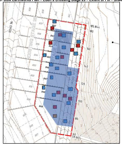
Figure 3: Bulk Earthworks Plan - Eden's Crossing Stage 29 - Extent of Fill - Shaded Blue
