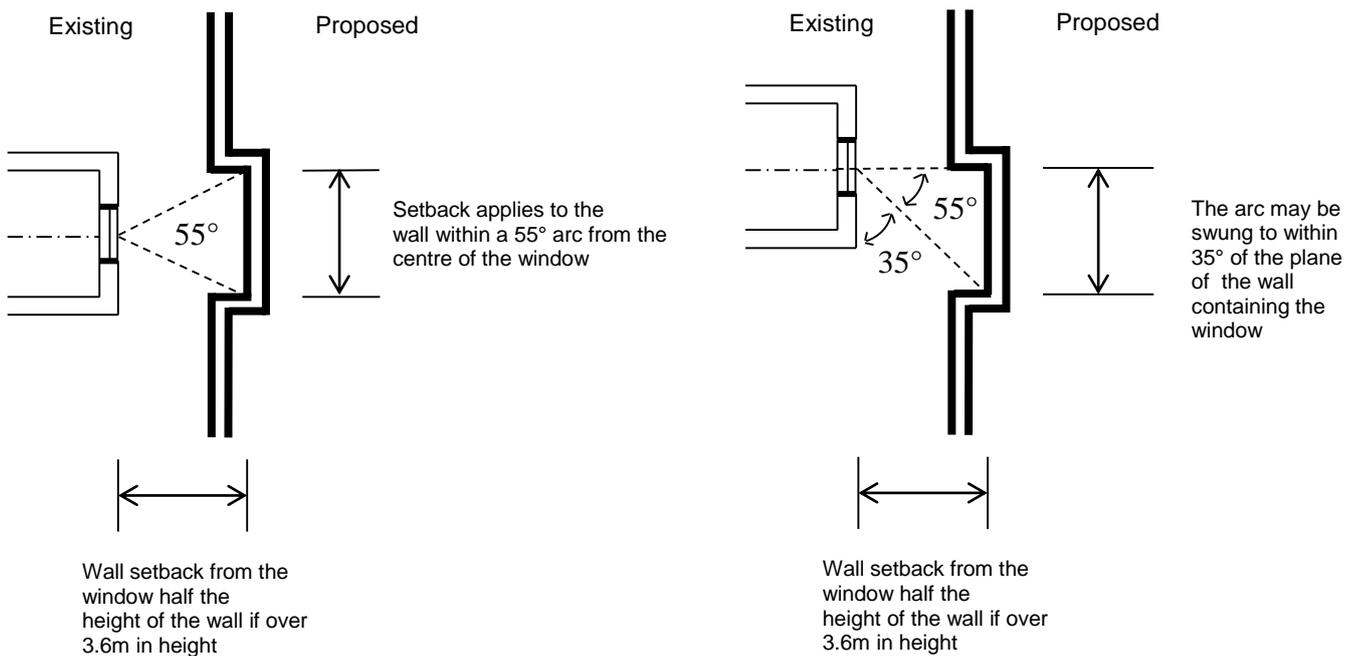
If the existing habitable room window is above ground level, the wall or carport height is measured from the floor level of the room containing the window.
