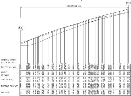
RETAINING WALL - LONGITUDINAL SECTION HORIZONTAL SCALE 1:500 @ A1 VERTICAL SCALE 1:50 @ A1
