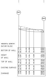
RETAINING WALL - LONGITUDINAL SECTION HORIZONTAL SCALE 1:500 @ A1 VERTICAL SCALE 1:50 @ A1
