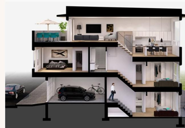
Split levels can account for the height difference between the front and rear of the allotment, without requiring extensive earthworks and reduce the visual prominence of multiple retaining walls.
