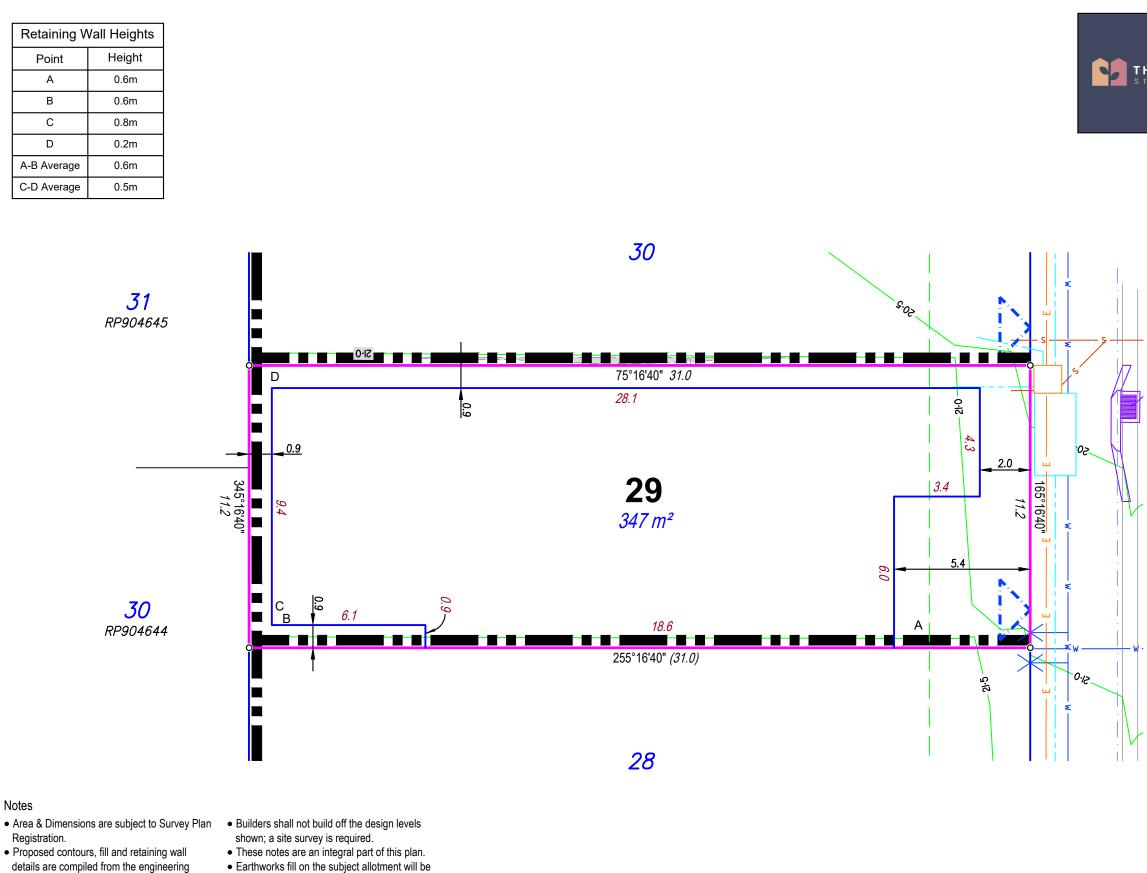
design plans provided by Peak Urban, undertaken and compacted in accordance with the provisions of AS3798-2007 Tables 5.1 and • Due to plotting limitations the retaining walls 8.1 under Level1 supervision. shown are indicative only and may not show
