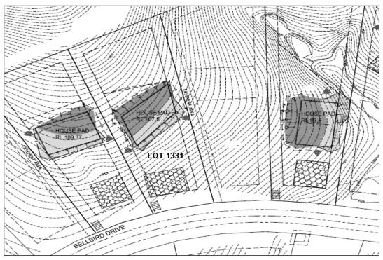
Approximate lateral extent and maximum depth of controlled filling to 1.6m. Level 1 Certification is limited to within this area.
