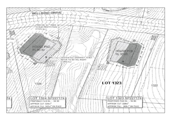
Approximate lateral extent and maximum depth of controlled filling to 1.5m. Level 1 Certification is limited to within this area.
