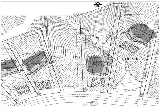
Approximate lateral extent and maximum depth of controlled filling to 1.5m. Level 1 Certification is limited to within this area.
