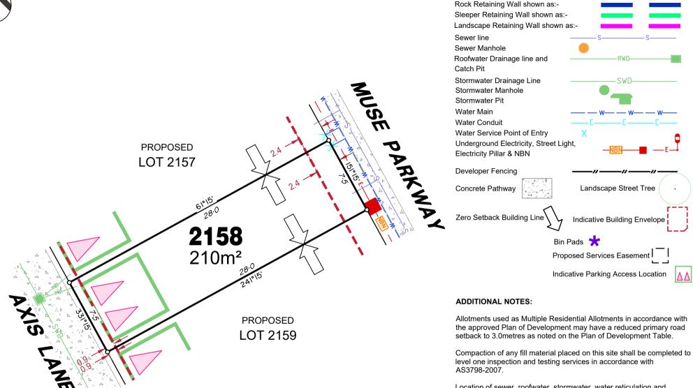
Location of sewer, roofwater, stormwater, water reticulation and electricity lines, manholes and pits are those shown on engineering design drawings, supplied by Colliers and may differ from the as-constructed location.
