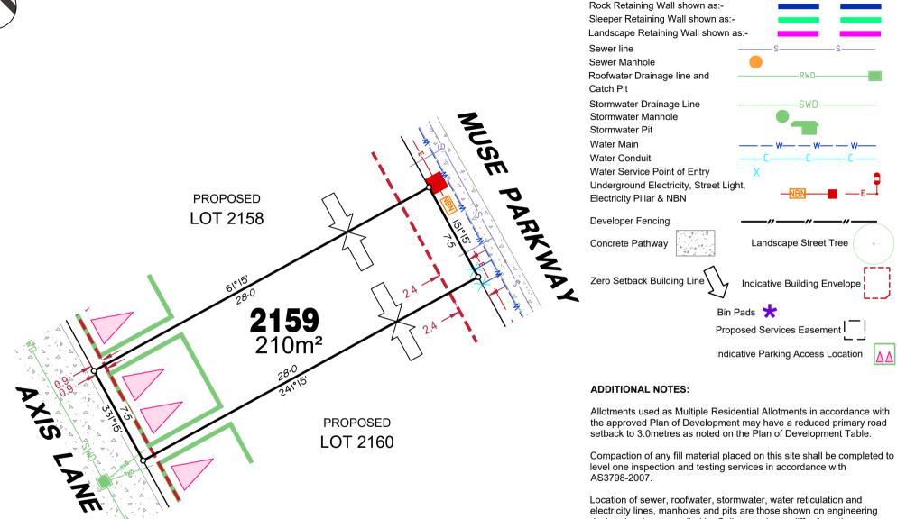
design drawings, supplied by Colliers and may differ from the as-constructed location.
