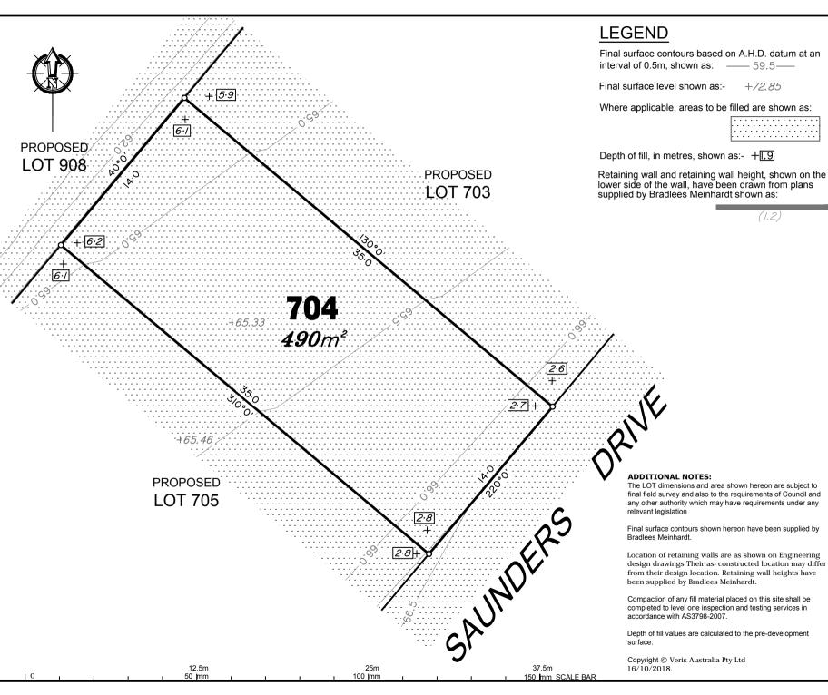
Final surface contours based on A.H.D. datum at an interval of 0.5m. shown as: ---- 59.5---
