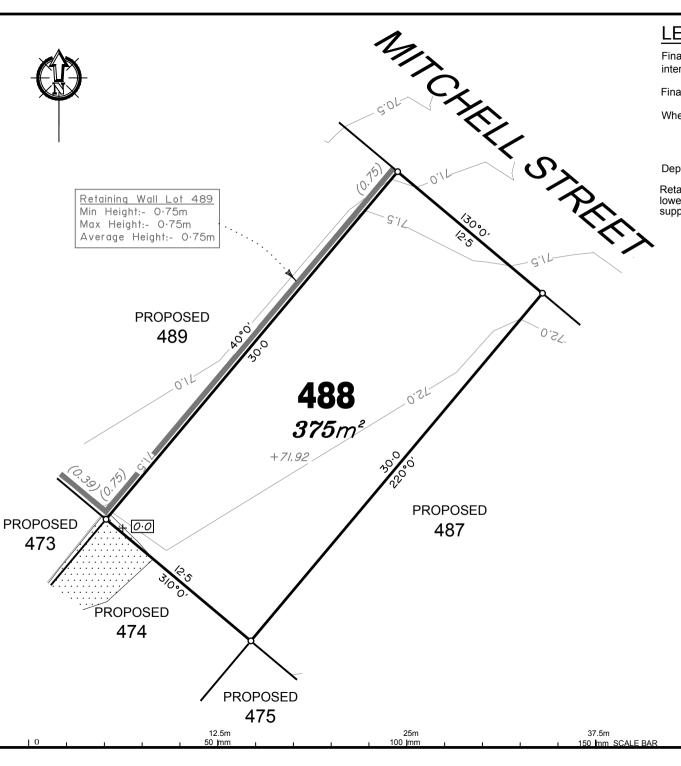
Final surface contours based on A.H.D. datum at an interval of 0.5m. shown as: ---- 59.5---
