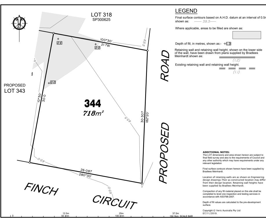
Final surface contours based on A.H.D. datum at an interval of 0.5m.
