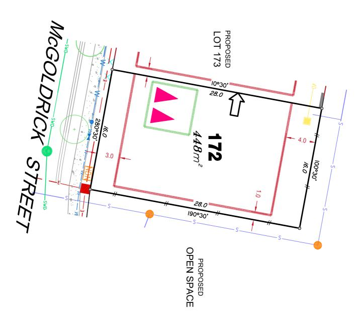
Proposed Services Easement Roofwater Drainage line and Retaining Wall shown as:-Electricity Pillar & NBN Stormwater Pit Stormwater Manhole Catch Pit Concrete Pathway Developer Fencing Underground Electricity, Street Light, Water Service Point of Entry Water Conduit Water Main Stormwater Drainage Line Sewer Manhole Sewer line Indicative Parking Access Location Zero Setback Building Line Indicative Building Envelope Landscape Street Tree
