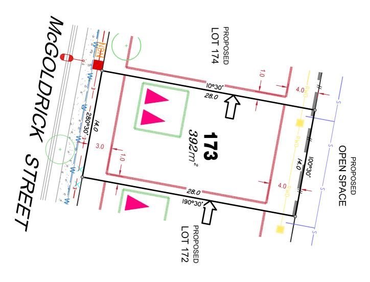
Proposed Services Easement Roofwater Drainage line and Retaining Wall shown as:-Stormwater Pit Stormwater Manhole Catch Pit Concrete Pathway Developer Fencing Electricity Pillar & NBN Underground Electricity, Street Light, Water Service Point of Entry Water Conduit Water Main Sewer Manhole Sewer line Indicative Parking Access Location Zero Setback Building Line Stormwater Drainage Line Indicative Building Envelope Landscape Street Tree
