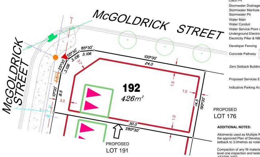
Retaining Wall shown as:-Sewer line Sewer Manhole Roofwater Drainage line and Catch Pit Stormwater Drainage Line Water Service Point of Entry Underground Electricity, Street Light, Electricity Pillar & NBN Landscape Street Tree Zero Setback Building Line Indicative Building Envelope Proposed Services Easement Indicative Parking Access Location
