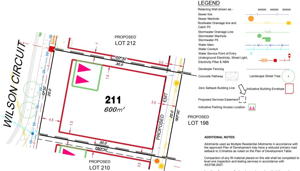
Location of sewer, roofwater, stormwater, water reticulation and electricity lines, manholes and pits are those shown on engineering design drawings, supplied by Bradlees Meinhardt, and may differ from the as-constructed location.
