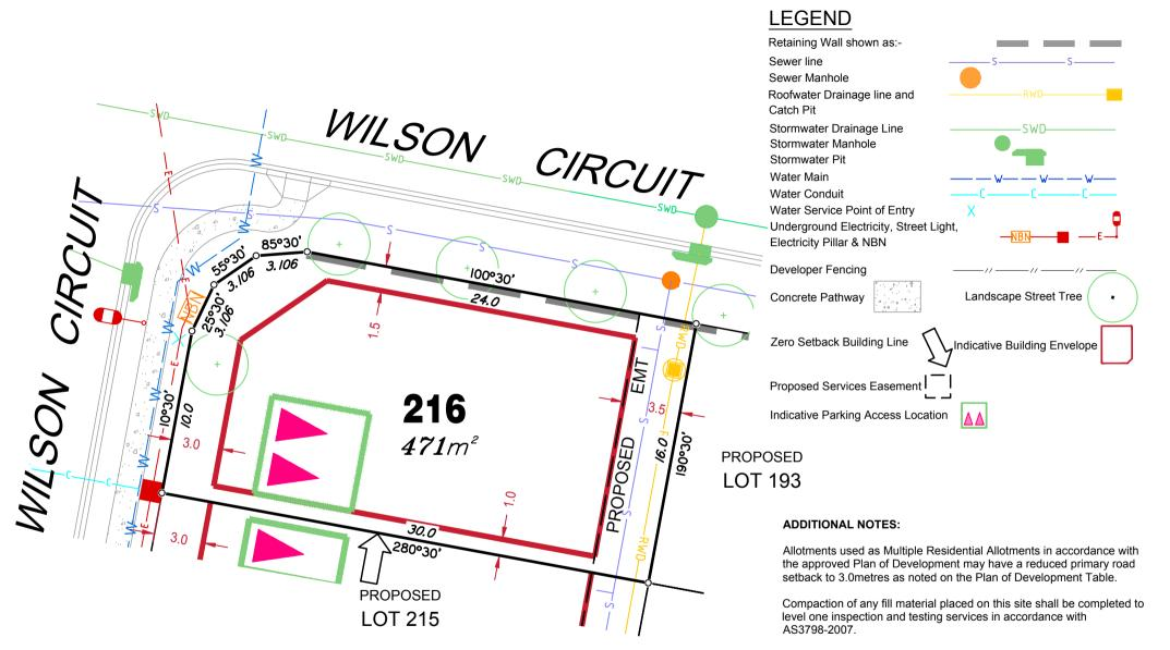
Location of sewer, roofwater, stormwater, water reticulation and electricity lines, manholes and pits are those shown on engineering design drawings, supplied by Bradlees Meinhardt, and may differ from the as-constructed location.
