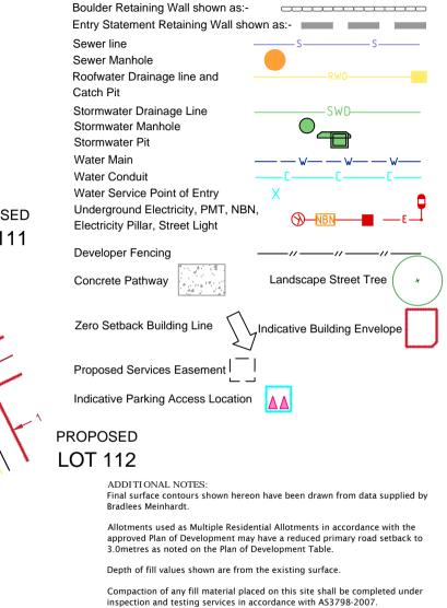
Location of sewer, roofwater, stormwater, water reticulation and electricity lines, manholes and pits are those shown on engineering design drawings, supplied by Bradlees Meinhardt, and may differ from the as-constructed location.
