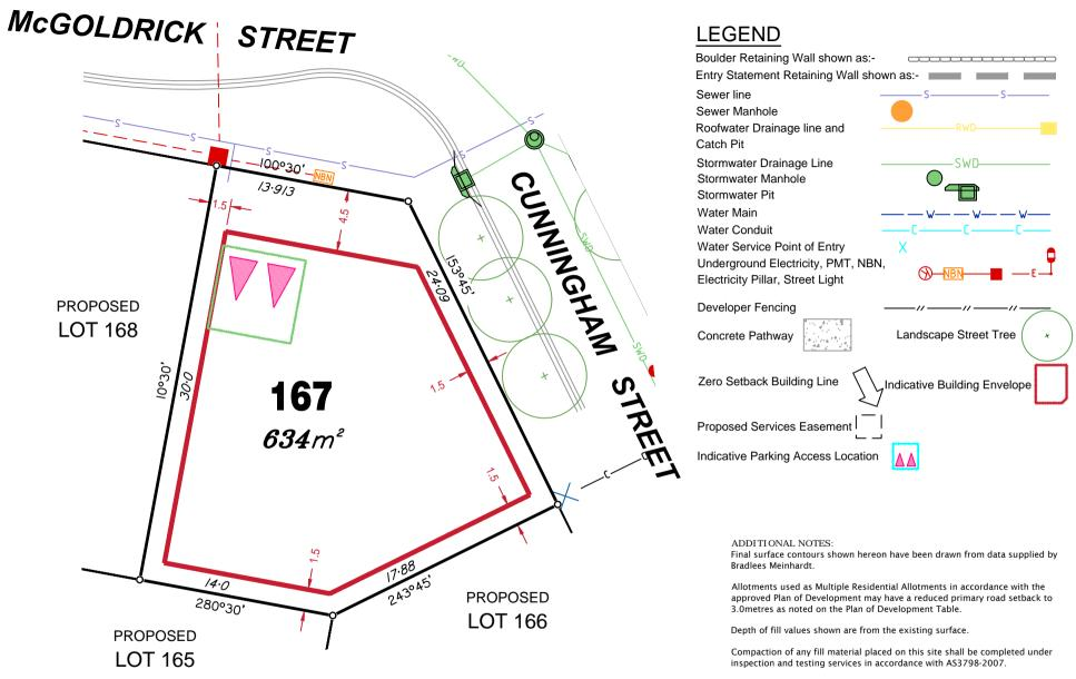
Location of sewer, roofwater, stormwater, water reticulation and electricity lines, manholes and pits are those shown on engineering design drawings, supplied by Bradlees Meinhardt, and may differ from the as-constructed location.
