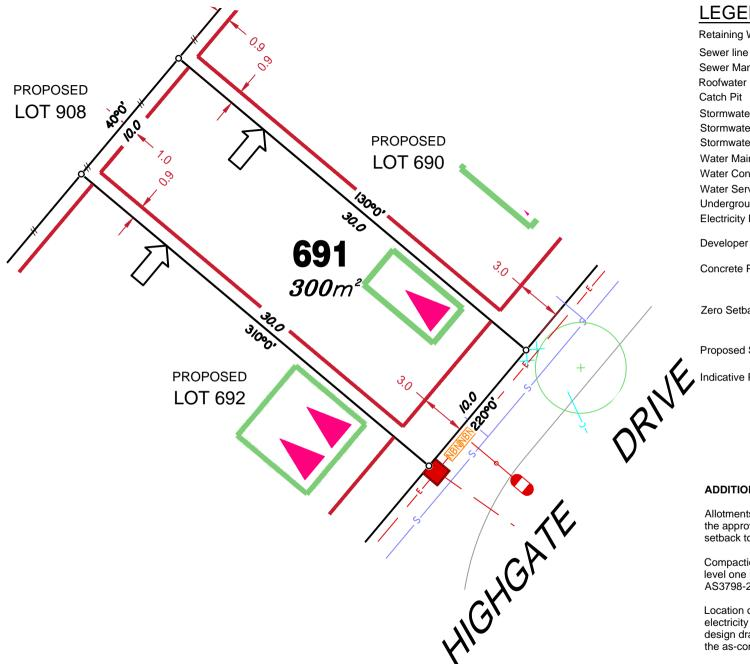
Retaining Wall shown as:-Sewer Manhole Roofwater Drainage line and Stormwater Drainage Line Stormwater Manhole Stormwater Pit Water Main Water Conduit Water Service Point of Entry Underground Electricity, Street Light, Electricity Pillar & NBN **Developer Fencing** Concrete Pathway Landscape Street Tree Zero Setback Building Line Indicative Building Envelope Proposed Services Easement Indicative Parking Access Location
