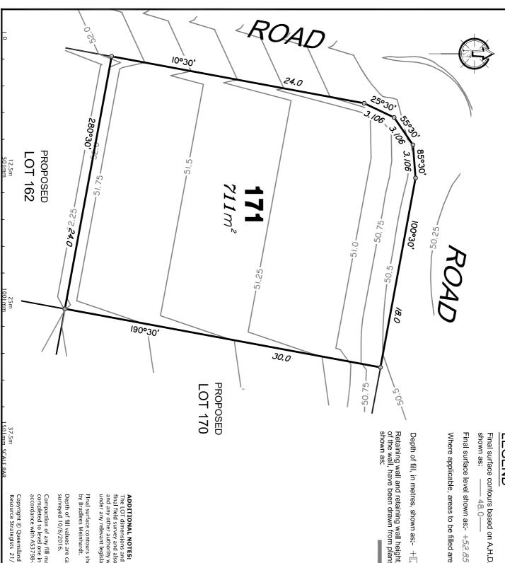
Final surface contours based on A.H.D. datum at an interval of 0.25m 48.0-
