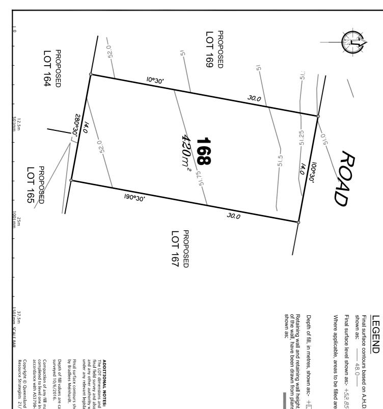
Final surface contours based on A.H.D. datum at an interval of 0.25m 48.0-
