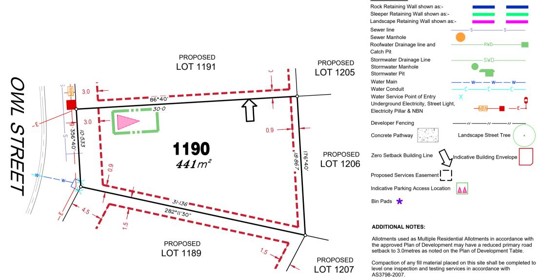
Location of sewer, roofwater, stormwater, water reticulation and electricity lines, manholes and pits are those shown on engineering design drawings, supplied by Peak Urban and may differ from the
