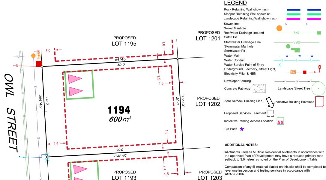
Location of sewer, roofwater, stormwater, water reticulation and electricity lines, manholes and pits are those shown on engineering design drawings, supplied by Peak Urban and may differ from the as-constructed location.
