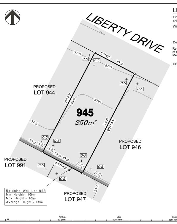
Final surface contours based on A.H.D. datum at an interval of 0.5m, shown as: —— 59.5——
