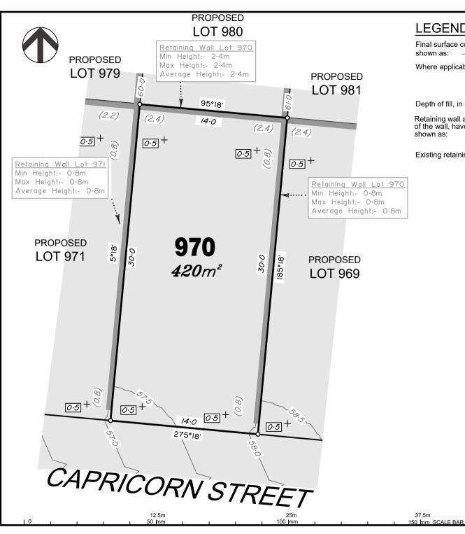
Final surface contours based on A.H.D. datum at an interval of 0.5m, shown as: —— .5.9..5——
