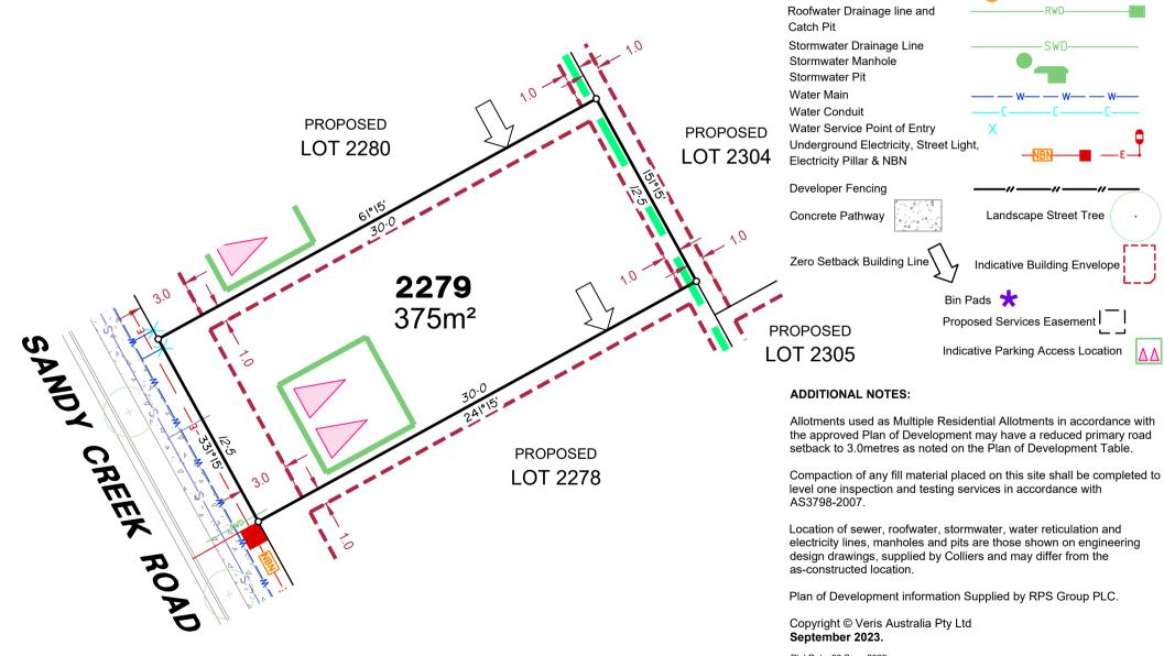
Rock Retaining Wall shown as:-Sleeper Retaining Wall shown as:-Landscape Retaining Wall shown as:-Sewer line Sewer Manhole Landscape Street Tree Indicative Building Envelope Proposed Services Easement
