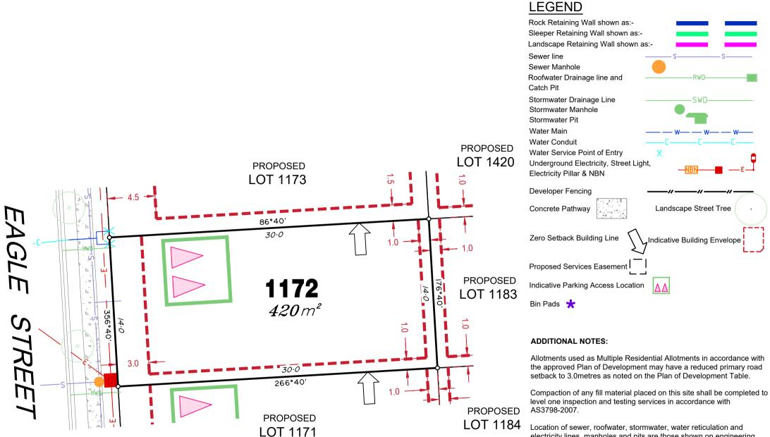
Location of sewer, roofwater, stormwater, water reticulation and electricity lines, manholes and pits are those shown on engineering design drawings, supplied by Colliers and may differ from the as-constructed location.
