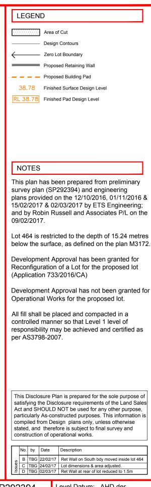
Level Datum: AHD der. Origin of Levels: PM161439 RL of Origin: 78.888 Contour Interval: 0.25m Scale @A3 1: 250 Dwg No. 8353 S 25 DP D 464
