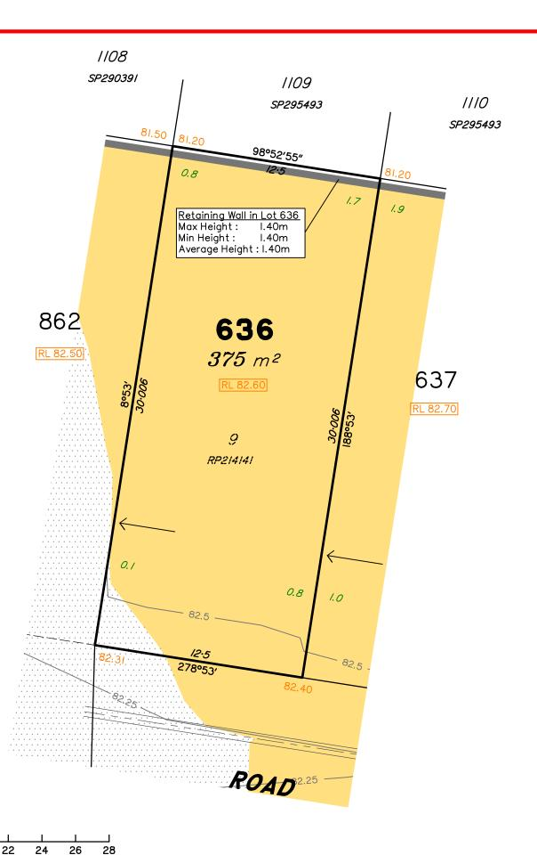
LEGEND Area of Fill Area of Cut Design Contours Zero Lot Boundary Retaining Wall 38.78 Finished Surface Design Level RL 38.78 Finished Pad Design Level (Not all items in this legend may be relevant to the lot
