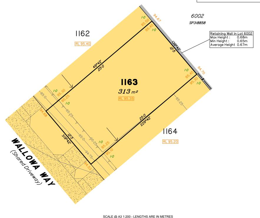
**LEGEND** Area of Cut Area of Fill **Design Contours** Depth of Fill Top of Batter Toe of Batter Preferred Pad Level Retaining Wall Finished Surface Design Level Optional Built to Boundary Wall Location 2.0m High Acoustic Fence (Not all items in this legend may be relevant to the lot shown)
