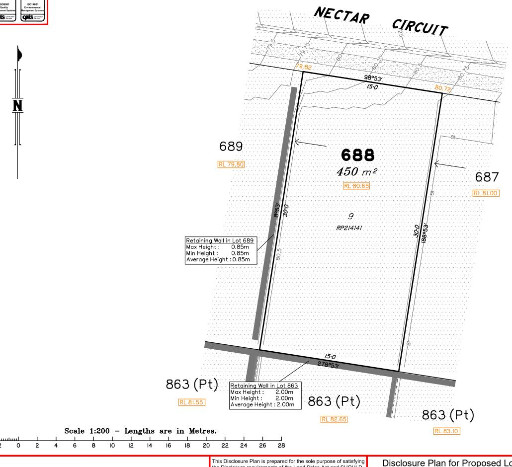
LEGEND Area of Fill Area of Cut **Design Contours**  Zero Lot Boundary Retaining Wall 38.78 Finished Surface Design Level RL 38.78 Finished Pad Design Level Depth of Fill
