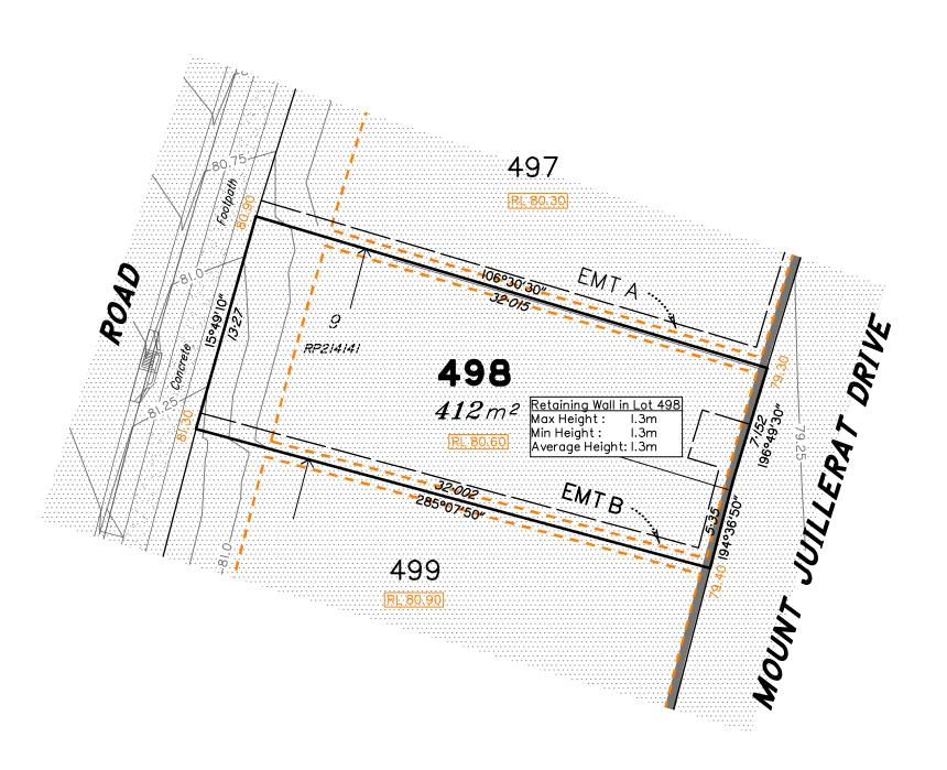
LEGEND Area of Cut **Design Contours** Zero Lot Boundary Proposed Retaining Wall Proposed Building Pad (Indicative) 38.78 Finished Surface Design Level RL 38.78 Finished Pad Design Level
