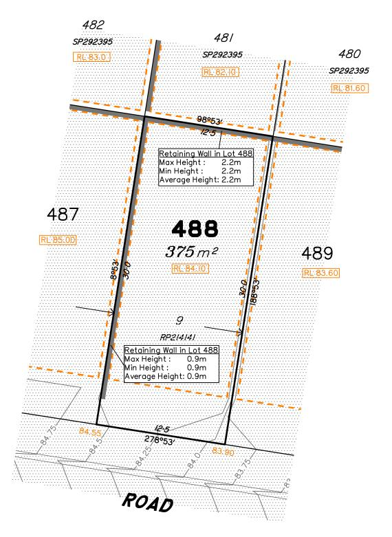
LEGEND Area of Cut Design Contours Zero Lot Boundary Proposed Retaining Wall Proposed Building Pad (Indicative) 38.78 Finished Surface Design Level RL 38.78 Finished Pad Design Level
