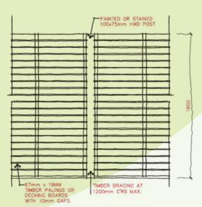
HORIZONTAL TIMBER WING FENCE SCALE 1: 20
