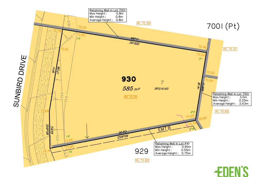
**LEGEND** Area of Cut Area of Fill **Design Contours** Depth of Fill Top of Batter Toe of Batter Retaining Wall Preferred Earthworks Pad Level Finished Surface Design Level Optional Built to Boundary Wall Sewer Line / Manhole Drainage Line / Pit
