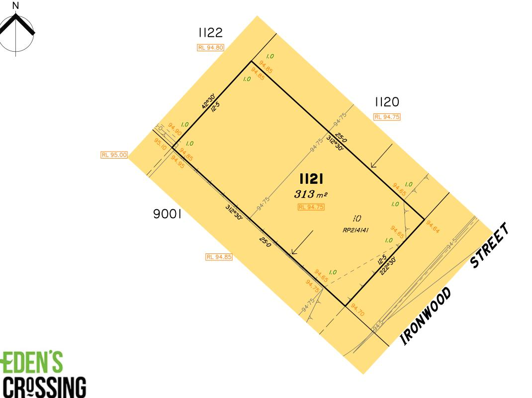
**LEGEND** Area of Cut Area of Fill **Design Contours** Depth of Fill Top of Batter Toe of Batter Preferred Pad Level Retaining Wall Finished Surface Design Level Optional Built to Boundary Wall Location
