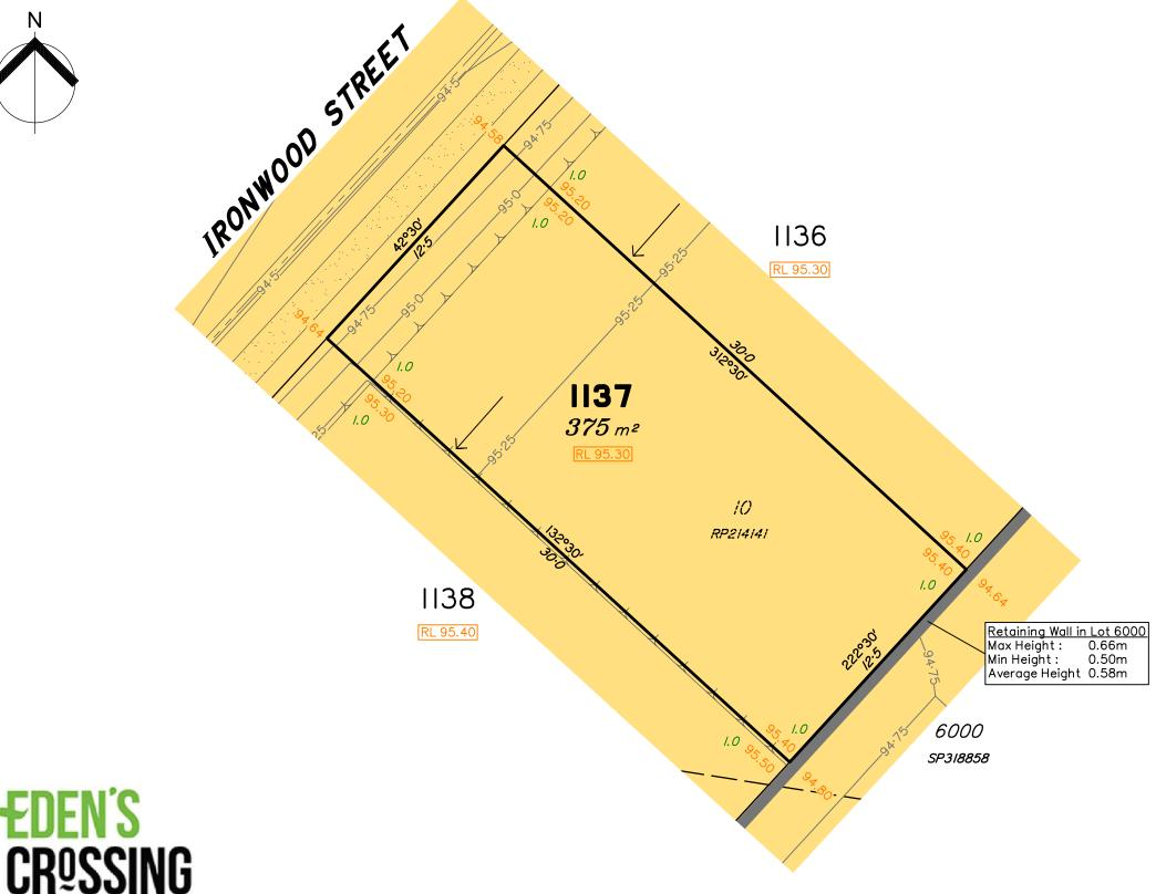
Area of Cut Area of Fill **Design Contours** Depth of Fill Top of Batter Toe of Batter Preferred Pad Level Retaining Wall Finished Surface Design Level
