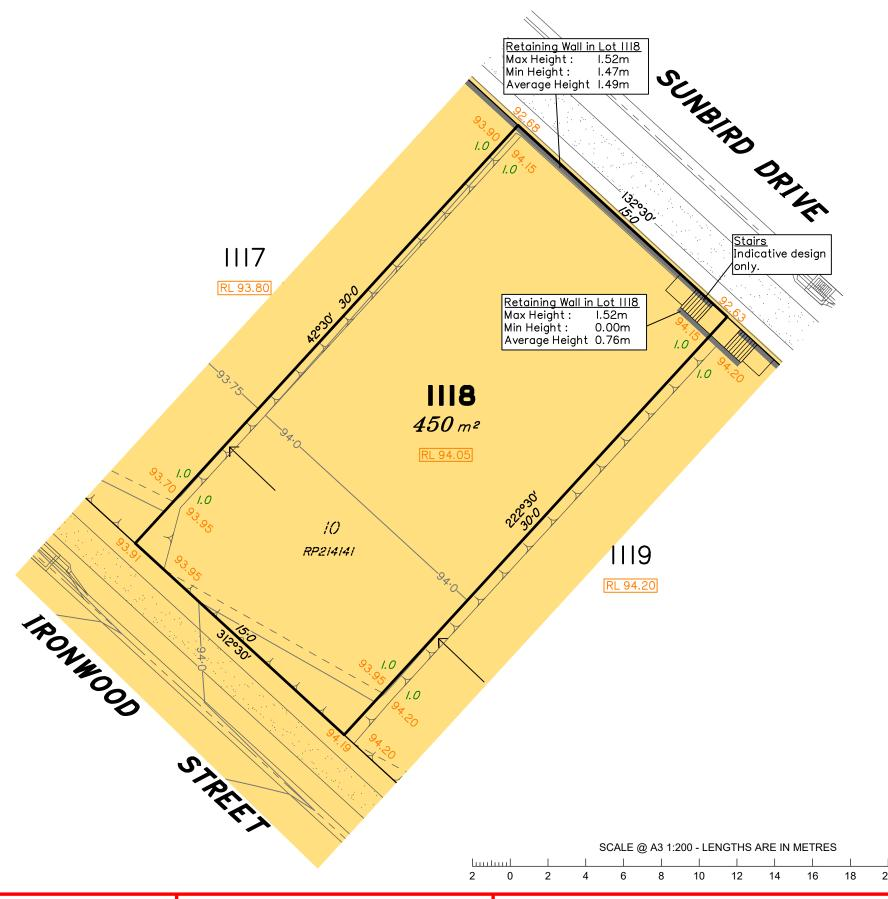
Area of Cut Area of Fill **Design Contours** Depth of Fill Top of Batter Toe of Batter Preferred Pad Level Retaining Wall Finished Surface Design Level
