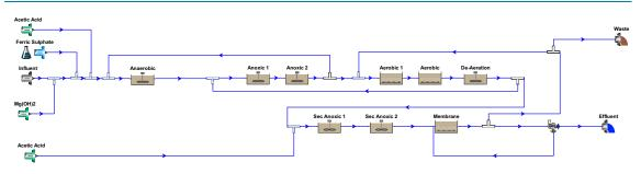
Figure 2-2 Googong WRP Flowchart (including Biological Phosphorus Removal)
