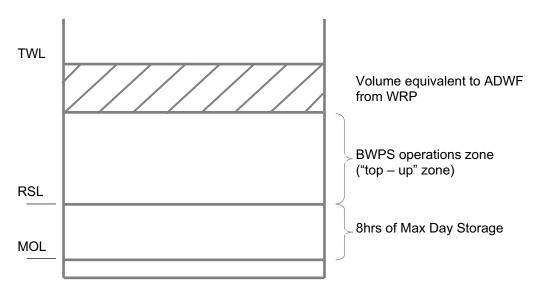
The schematic in Figure 4-1 shows key reservoir operating sections.
