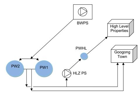
Figure 1-4 Schematic of Permanent Potable Water System (Whole Development)
