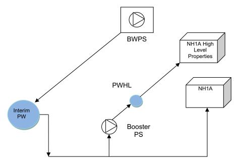
Figure 1-3 Schematic of Interim Potable Water Supply System (NH1A Only)
