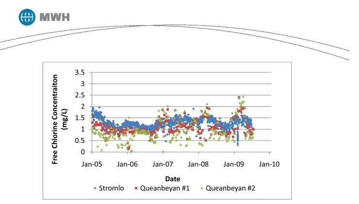
Figure B-2 Stromlo WTP and Queanbeyan Free Chlorine Concentrations
