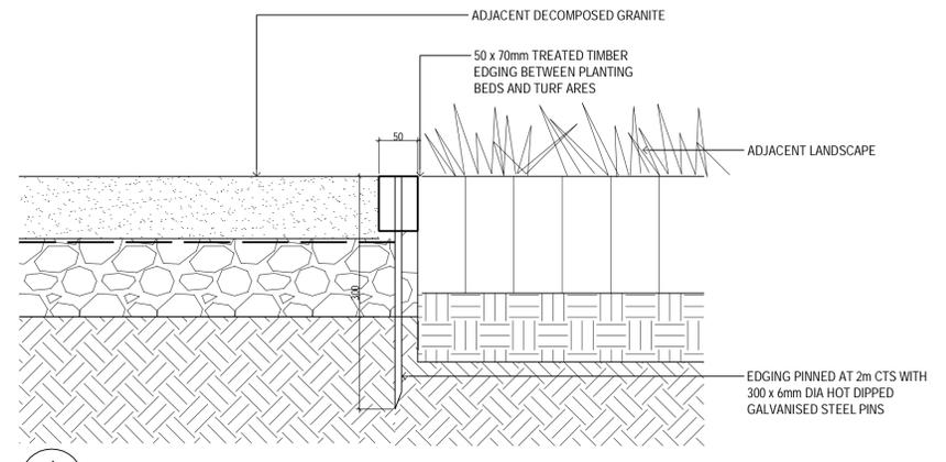
**4** PAVEMENT DETAIL 4: P5 DECOMPOSED GRANITE GRAVEL
