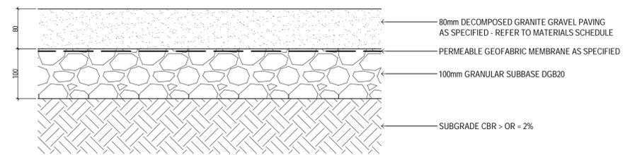
**3** PAVEMENT DETAIL 2: P2 DECOMPOSED GRANITE GRAVEL
